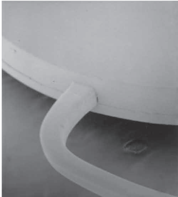
Scanning electron micrograph of the foldable silicone PCIOL (911, Pharmacia, Kalamazoo, MI) for implantation into the capsular bag. The sharp-edged optic shows small irregularities and molding flash (magnification \times 78.0 ).
